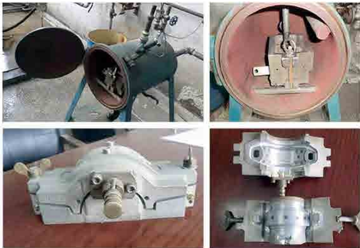
Figure 2.10 Steam cylinder forming equipment
