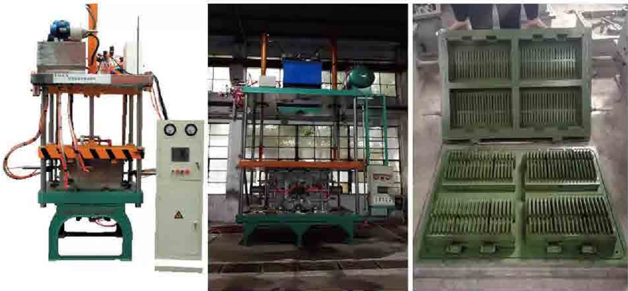
Figure 2.11 Press air chamber forming equipment
