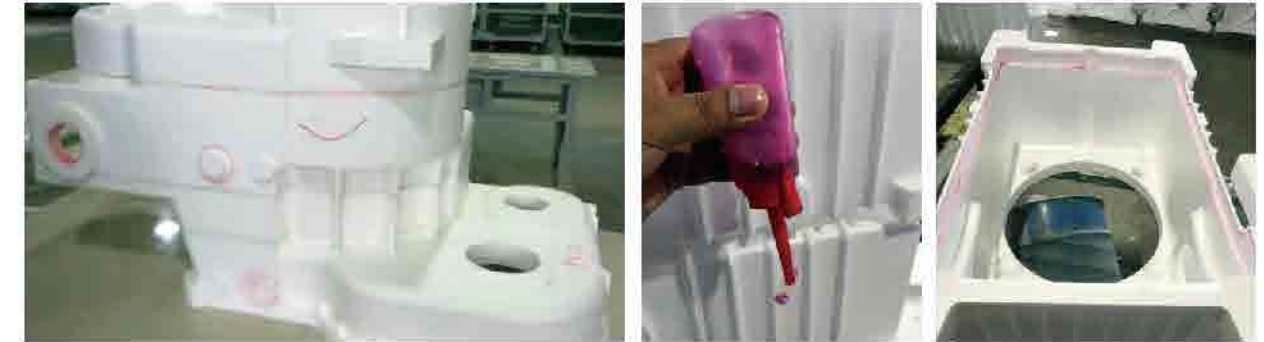
Figure 2.30 Schematic diagram of manual gluing
