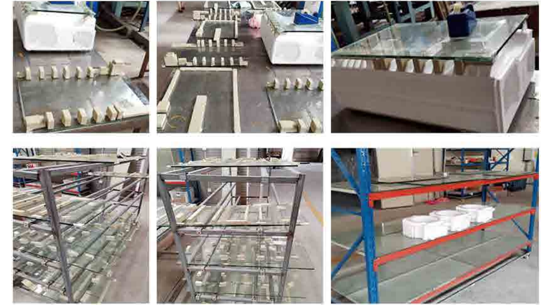
Figure 2.27 Special mold drying rack
