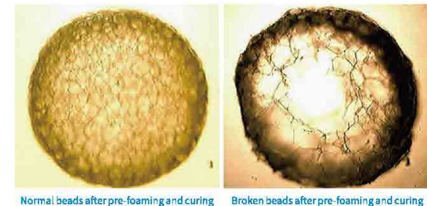
Figure 2.9 Beads after curing
